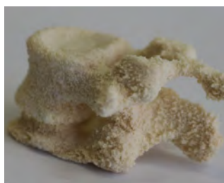
3D printed vertebra made of ethylcellulose, printed using solvent jetting
