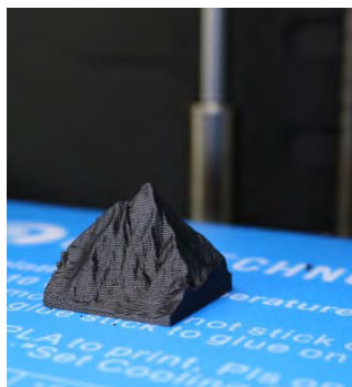
FDM printing of Matterhorn, PVB with 15% w/w CNT
