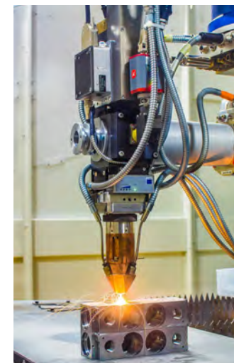
Lasercladding process for efficient coating against wear and corrosion
