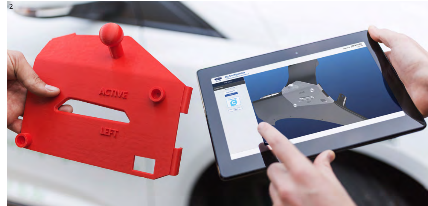
1 Configurator for the automated design of positioning jigs
