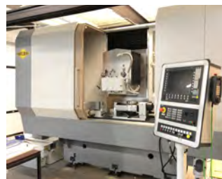
Hybrid machine for Laser Metal Deposition (LMD) and machining
