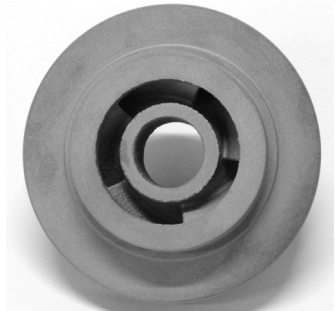
Pump impeller designed and produced by SLM at IPPE (project funded by CTI/Innosuisse)
