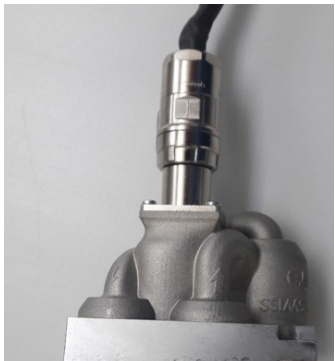
Intelligent H2-valve with integrated sensors for condition monitoring
